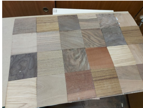
Picture 14: Cajon drums frame and glued veneers for decorative front panel.
