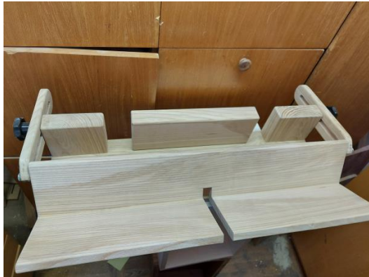
Picture 3: The production of drums required a special template, created for this purpose.
